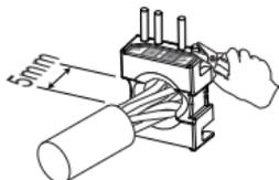
Insert a cable into the termination cap and fan out all four twisted pairs.
