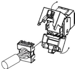
Install the termination cap to outlet, which will also allocate the conductors sitting on the slots.
