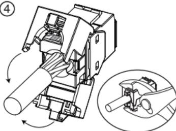
Secure the hinged outlet by using a crimp tool until it completely snap to effect the connection.
