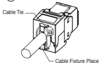
Fasten a cable tie wrap to secure the cable fixture place
